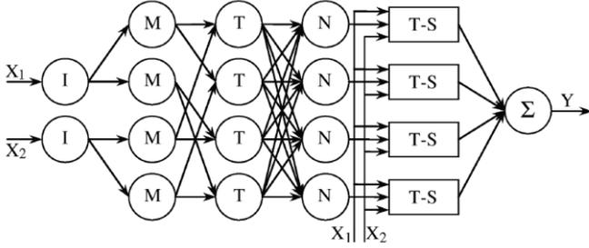
Fig. 2. A sample neurofuzzy structure equivalent with a MISO TSK fuzzy inference system
