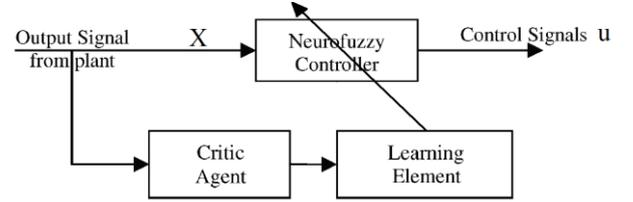
Fig. 3. Structure of adaptive critic-based neurofuzzy controller(ACNFC)
