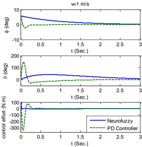
Fig. 6. Initial Response of Bicycle at  $v=1\text{m/s}$  a) Roll angle, b) Steer angle and c) control effort
