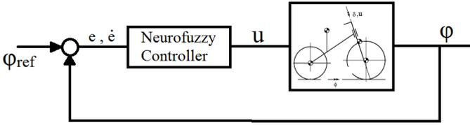
Fig. 4. Structure of ACNFC for bicycle
