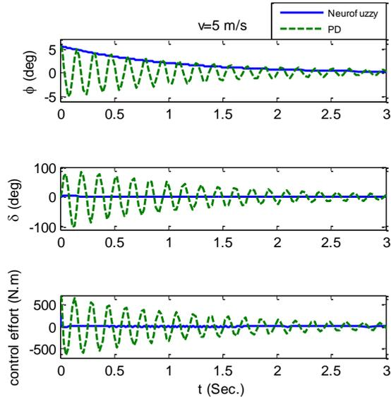
Fig. 7. Initial Response of Bicycle at  $v=5\text{m/s}$  a) Roll angle, b) Steer angle, c) Control effort
