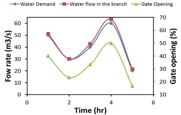
Fig. 9: Optimal gate opening - Scenario 1
