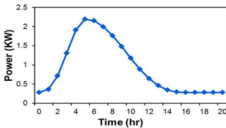
Fig. 8: Variation of turbine power with time
