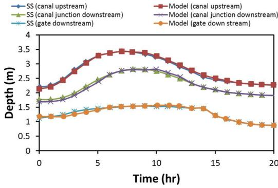
Fig. 6: Depth profile - Integrated model
