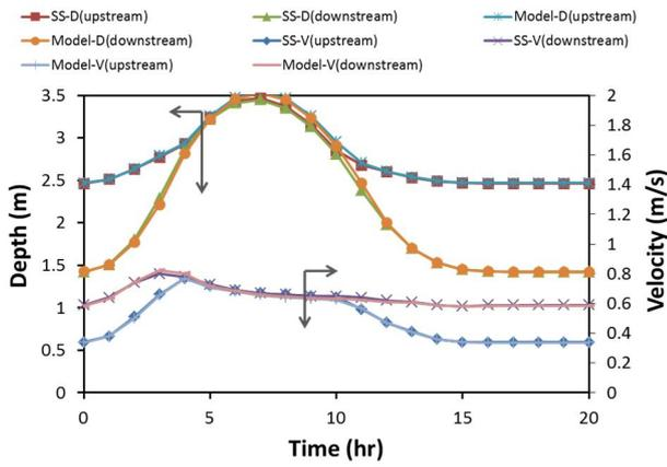
Fig. 2: Depth and velocity profiles - Canal weir
