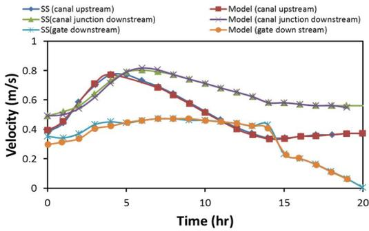
Fig. 7: Velocity profile - Integrated model
