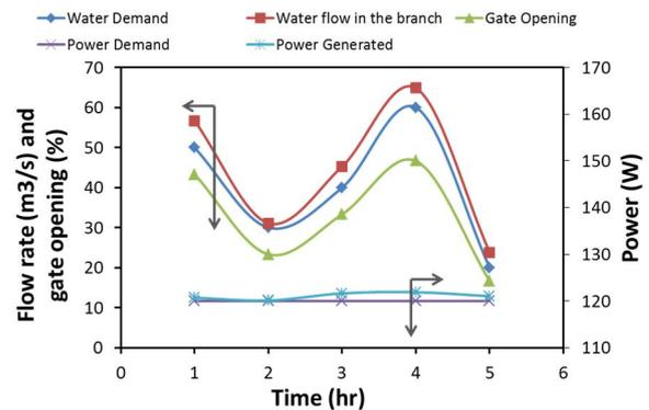
Fig. 10: Optimal gate opening - Scenario 2
