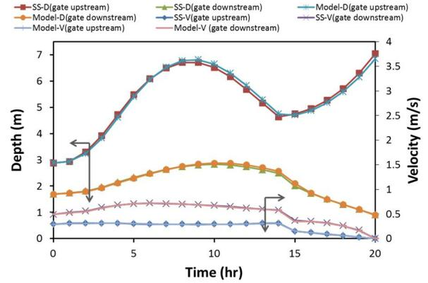
Fig. 4: Depth and velocity profiles - Canal gate
