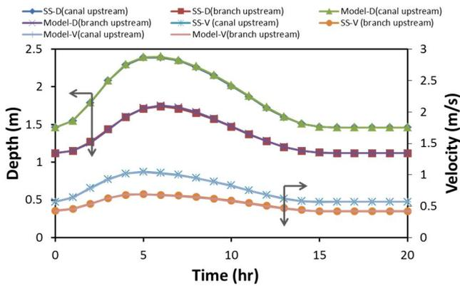
Fig. 3: Depth and velocity profile - Canal junction
