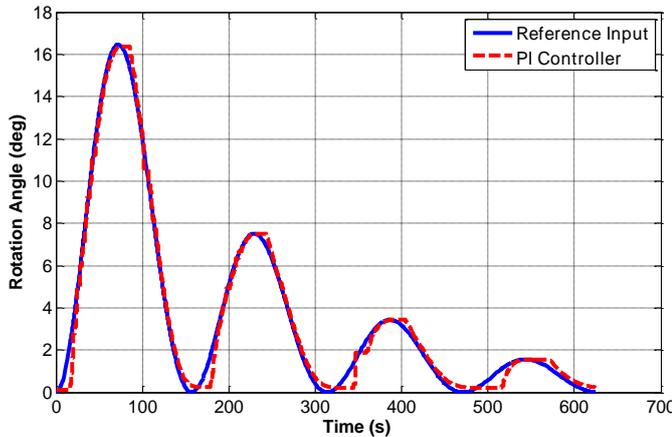
Fig. 16. Tracking control of a decaying sinusoidal wave.
