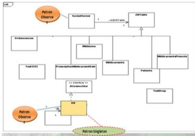
Fig. 8. The extraction component and its associated patterns.
