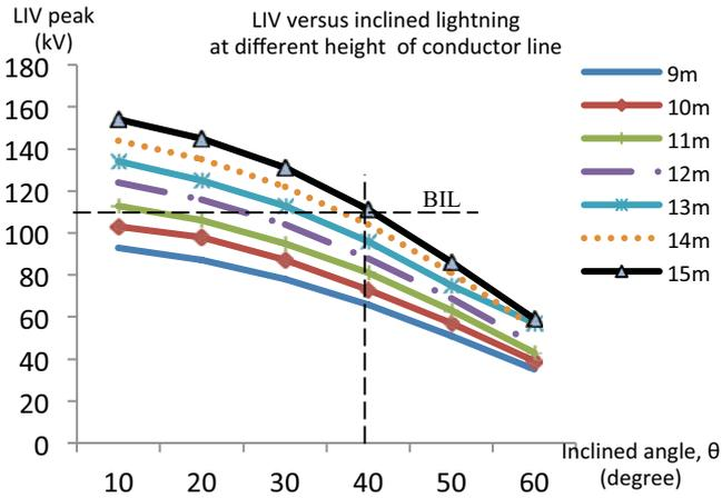
Fig 3. The behaviour of the LIV for variation of inclined angle and height of conductor (at  $\phi=70^\circ, v = 1.5 \times 10^8 \text{ m/s}, d=50\text{m}$ )
