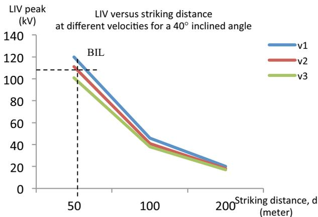
Fig. 7 The behaviour of the LIV on variation of striking distance and velocity return stroke at a specific inclined angle (at  $\phi=70^\circ$ ,  $\theta=40^\circ$ ,  $h=15$ m,  $v_1=1.2 \times 10^8$  m/s,  $v_2=1.5 \times 10^8$  m/s,  $v_3=1.9 \times 10^8$  m/s)
