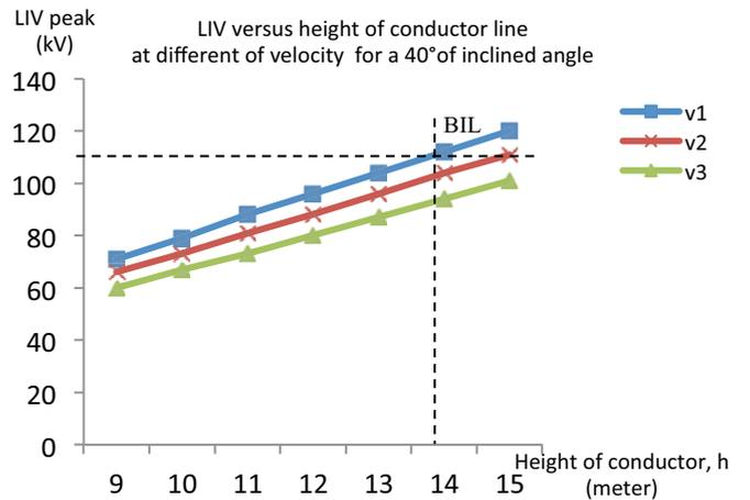
Fig.5 The behaviour of the LIV for variation of height of conductor and velocity of return stroke at specific inclined angles (at  $\phi=70^\circ, \theta= 40^\circ, d=50\text{m}, v1=1.2 \times 10^8 \text{ m/s}, v2=1.5 \times 10^8 \text{ m/s}, v3=1.9 \times 10^8 \text{ m/s}$ )
