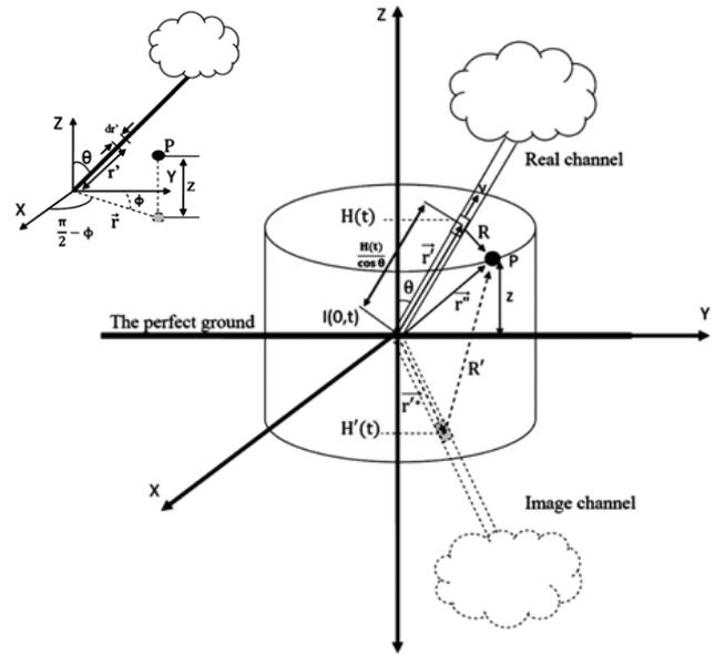
Fig. 2. Problem geometry for evaluating the electromagnetic field due to an inclined lightning channel [22, 26].
