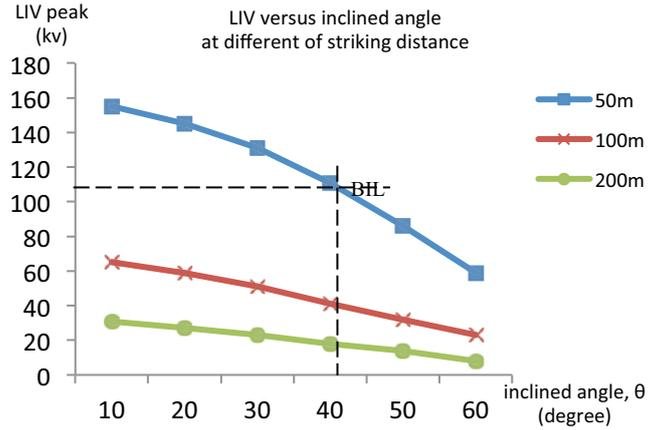
Fig 4. The behaviour of the LIV for variation of inclined angle and striking distance at specific of height of conductor (at  $\phi=70^\circ, v = 1.5 \times 10^8 \text{ m/s}, h=13.48\text{m}$ )
