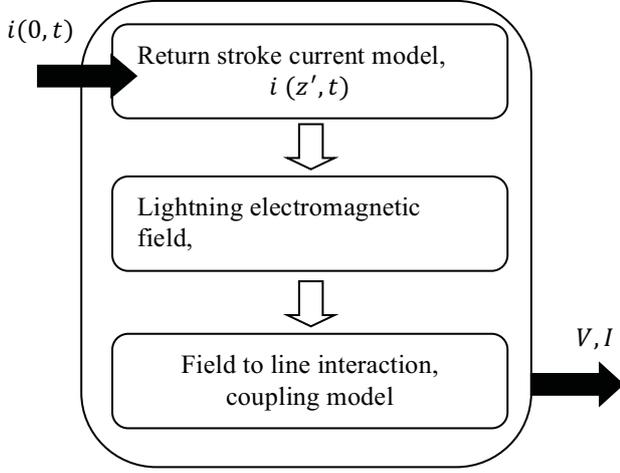
Fig.1 Block diagram for calculating the lightning induced voltage.[25]
