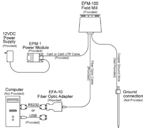
Figure 1: EFM-100 Connection Diagram
