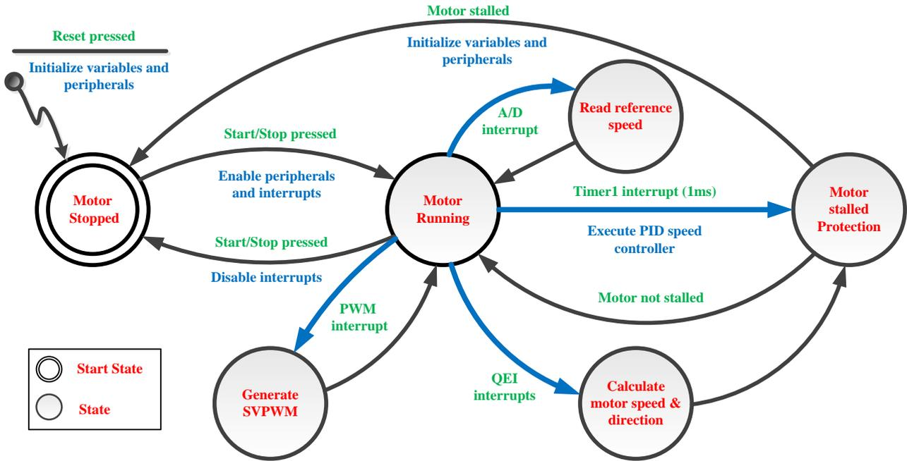
Fig. 6. Finite state machine
