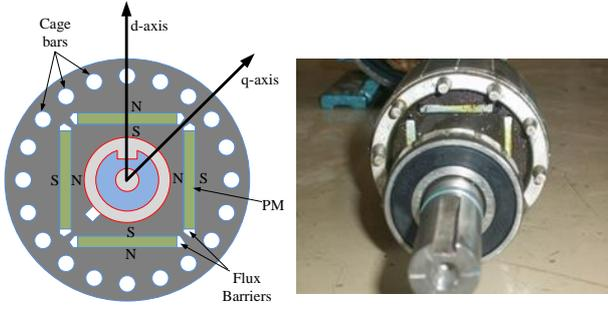
Fig. 2. Line start IPMSM rotor structure
