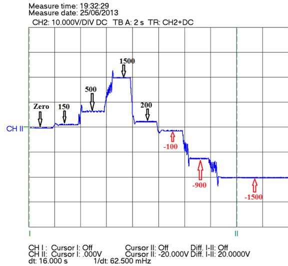
Fig. 13. Speed profile over a wide speed range in both directions of rotations
