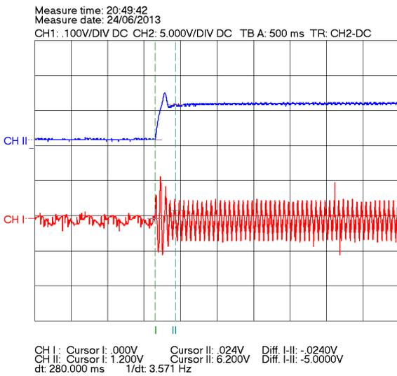
Fig. 11. Speed change from 150 r/min to 500 r/min
