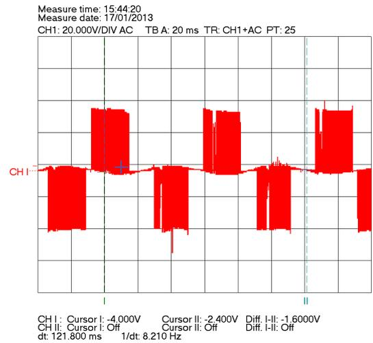
Fig. 9. Sample of measured line-line voltage
