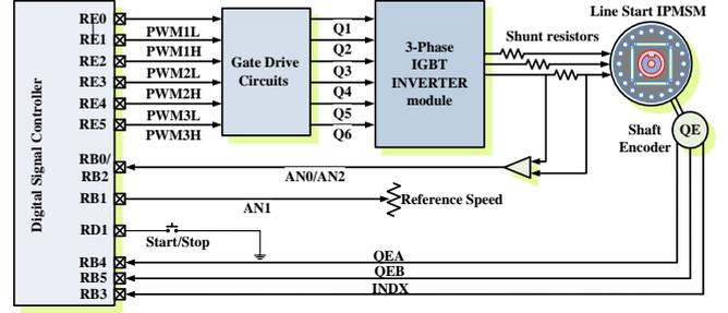
Fig. 3. Closed loop speed control system
