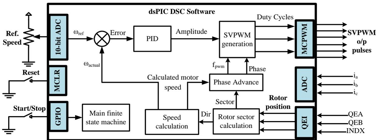
Fig. 5. Control System Design
