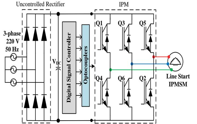
Fig. 4. Power Circuit
