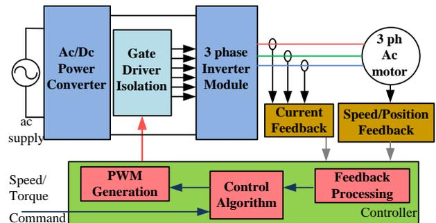
Fig. 1. Variable frequency drive system
