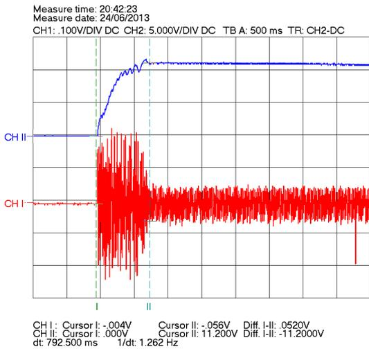
Fig. 10. Starting from standstill to rated speed (2A/div)
