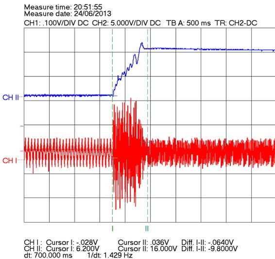
Fig. 12. Speed change from 500 r/min to 1500 r/min
