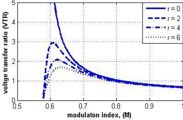
Fig. 5. Voltage transfer ratio versus modulation index for different inductor resistance for MCB control technique
