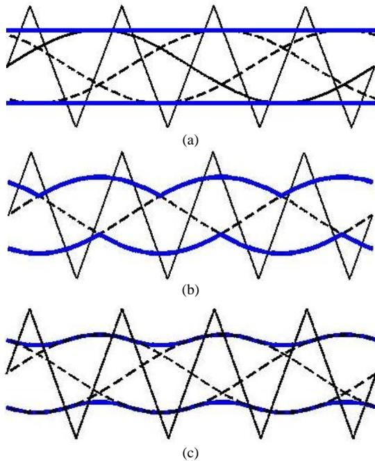
Fig. 2. Modulation schemes (a) SB, (b) MB and (c) MCB
