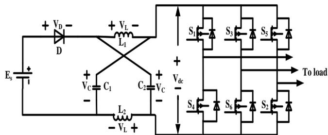
Fig. 1. Three-Phase Z-Source Inverter
