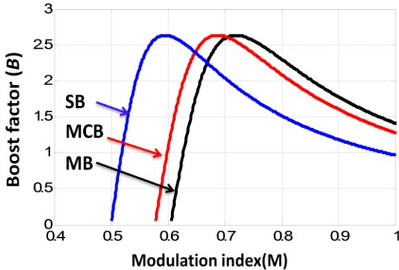
Fig. 6. Boost factor versus modulation index considering and neglecting inductor internal resistance “ $r$ ”
