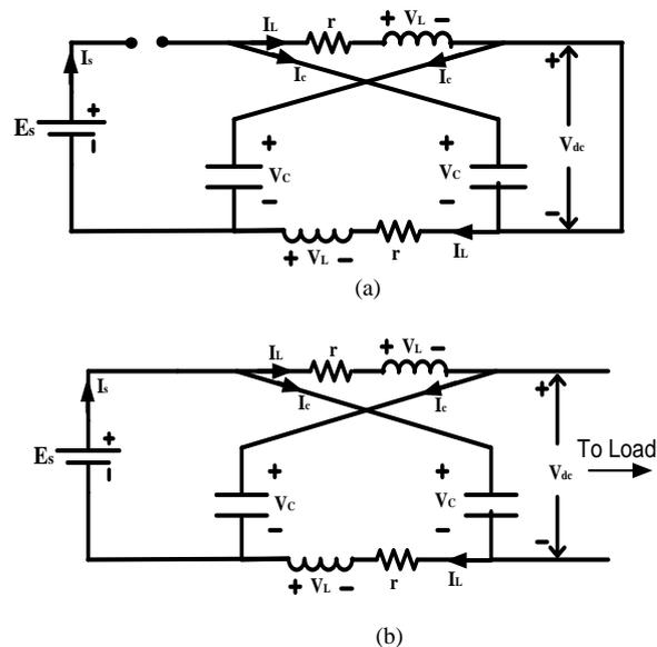
Fig. 3. Equivalent circuit of the Z-source inverter (a) Shoot-through state (b) Non shoot-through state.
