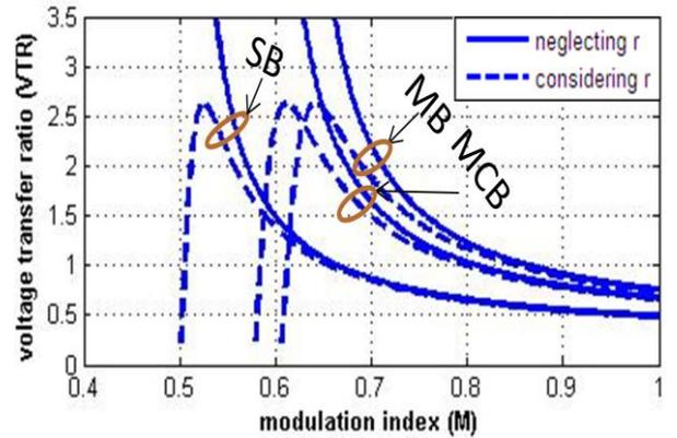
Fig. 4. Voltage transfer ratio versus modulation index considering and neglecting inductor internal resistance "r" where  $r=2.5\Omega$
