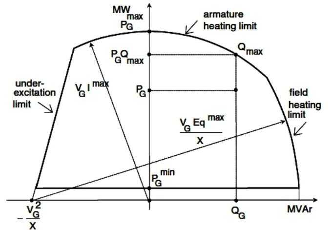
Figure 1. Capability curve of synchronous generator
