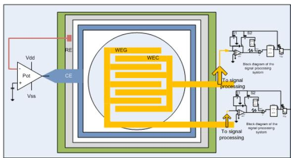
Fig. 6. The Fully Label-free impedimetric immunosensor chip.
