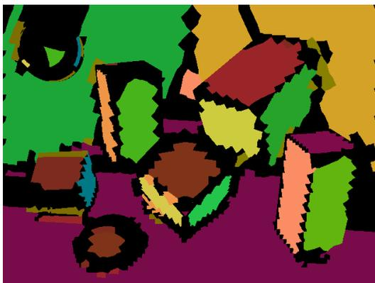
Fig. 6. Reconstructed, segmented normal direction image, 44 layers, steep regions were omitted
