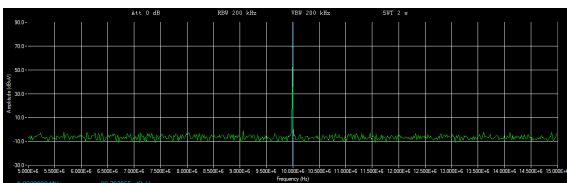
Fig. 5. AM-modulated chirp signal in 10 MHz.
