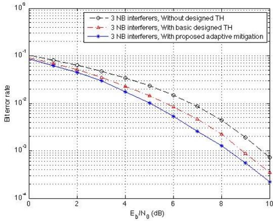
Figure 5. The BER of an UWB system with and without the designed TH sequence, in the presence of three NB interferers at  $f_1=2.402$  GHz,  $f_2=2.41$  GHz and  $f_3=2.42$  GHz with time-varying amplitudes.
