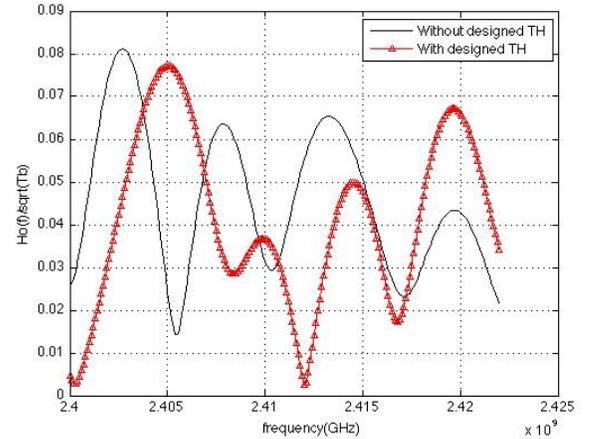
Figure 4. Normalized transfer function of the matched filter with and without the TH code design in the presence of single NB interferer at  $f_n = 2.412$  GHz.
