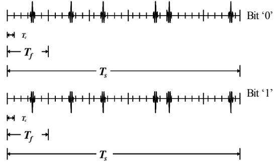
Figure 2. The transmitted DS-TH UWB signal at  $N_s=6$  and  $N_b=4$ .
