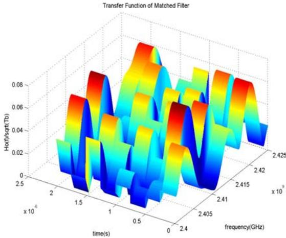
Figure 6. 3-D plot of time vs. frequency vs. normalized MF transfer function shows the adaptive multi-NB interferences mitigation.
