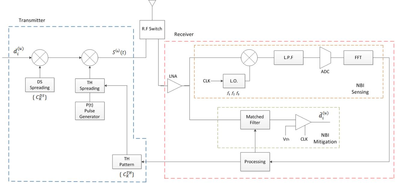
Figure 3. The proposed Adaptive mitigation UWB transceiver
