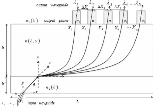
Figure 1. Geometry of the N-channel CWDM demultiplexer.
